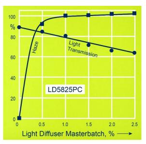
Even small amounts of masterbatch cause efficient light scattering in originally transparent polycarbonate.
